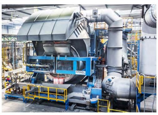
Tilting drum melting furnace
