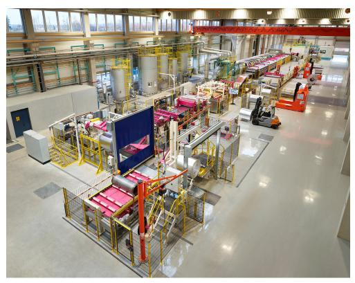
With the new surface treatment line at the Ranshofen site, our high-quality aluminium coils can be optimally prepared for further processing by the customer. Equipped with state-of-the-art technology, this plant enables the flexible surface finishing of different products and therefore offers advantages for customers from several industries.
