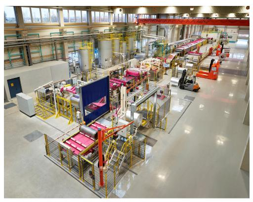
With the new surface treatment line at the Ranshofen site, our high-quality aluminium coils can be optimally prepared for further processing by the customer. Equipped with state-of-the-art technology, this plant enables the flexible surface finishing of different products and therefore offers advantages for customers from several industries.
