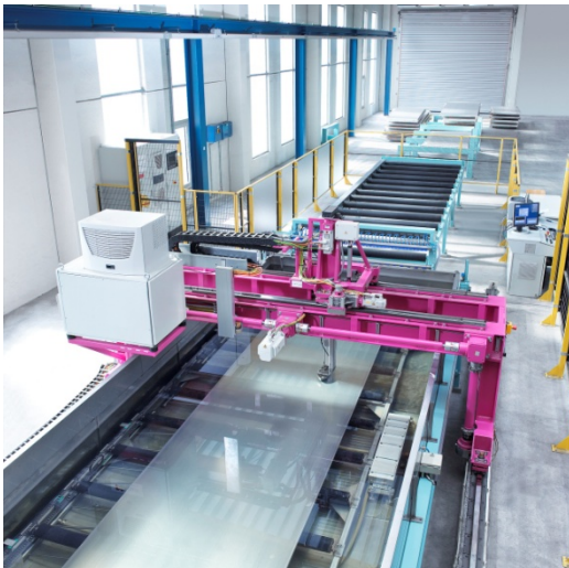
Picture 1: Testing technology at highest level: The demands made on testing technology have undergone a permanent increase due to the sophisticated applications in the aerospace industry. Picture showing AMAG aerospace plates at the ultrasonic inspection line where quality testing is completed several times more quickly.
