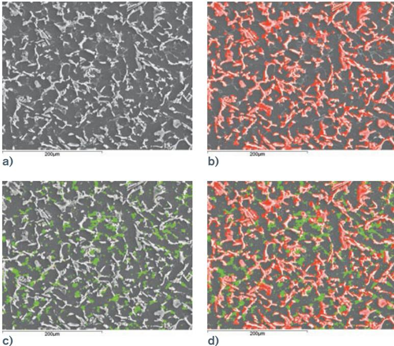
**Figure 1: SEM Depiction of the Si-Ni Network of an AlSi7Ni1.5 alloy after deep etching, without mapping (a), Si-mapping (b), Ni-mapping (c), Si-Ni mapping (d)**
