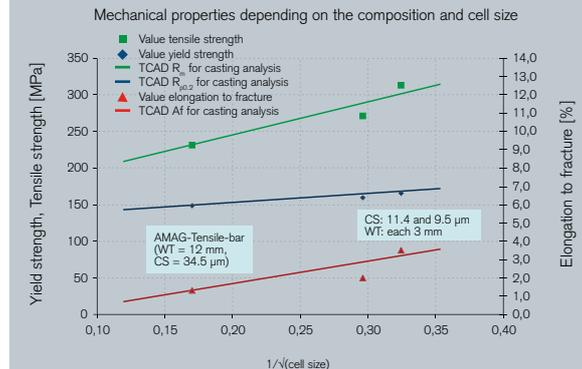
**Fig. 3:** Mechanical properties of high pressure die cast part – car oil pan
