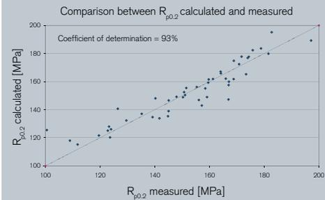
**Fig. 1:** Calculation model for yield strength, comparison of measured and corresponding calculated values
