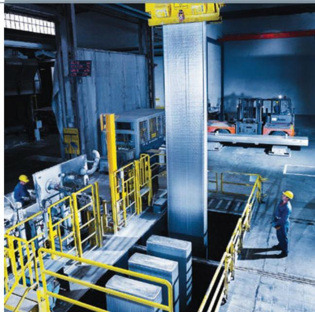
Removal of the ingots from the casting pit
