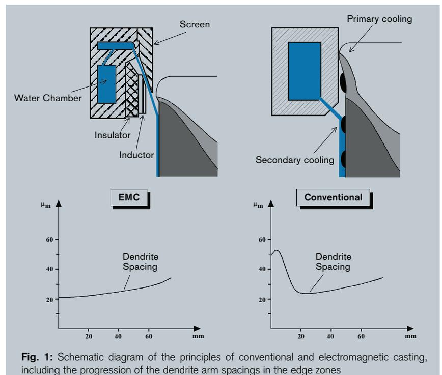
**Fig. 1:** Schematic diagram of the principles of conventional and electromagnetic casting, including the progression of the dendrite arm spacings in the edge zones
