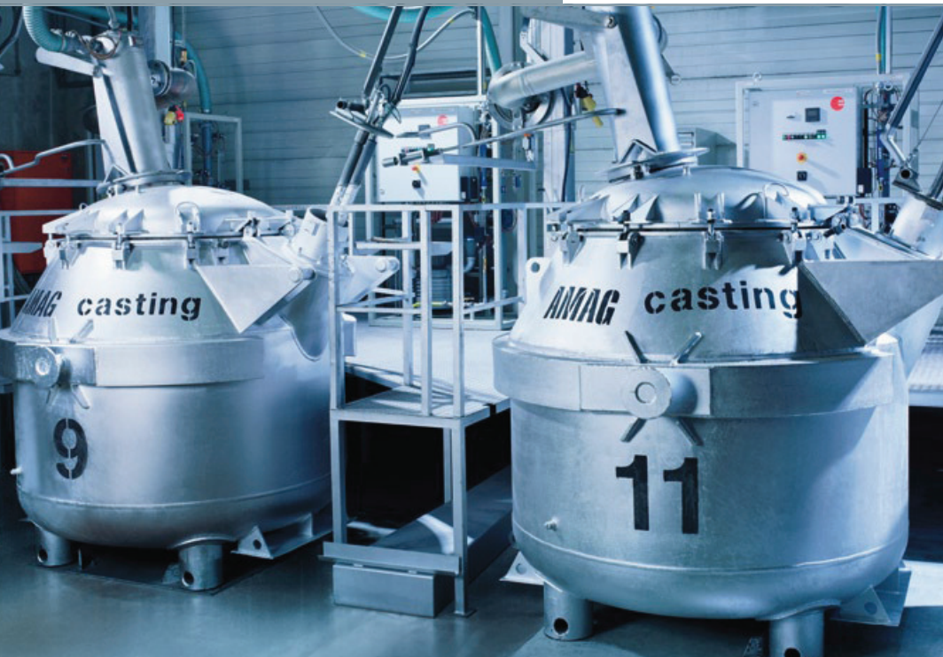
The heating of road transport ladles by means of gas burners
