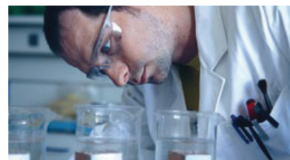
Abb.: ASSET Test (Test Method of Visual Assessment of Exfoliation Corrosion Susceptibility) gemäß ASTM G66
