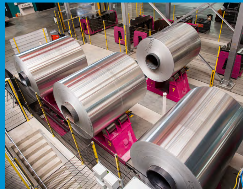
Strips with a width of over two meters in the coil preparation unit of the new cold rolling mill
